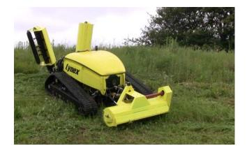
The powerful transmission sits in closed well tested gearboxes. We've only used the best components to ensure the highest possible efficiency. If the machine is equipped with a hydraulic shredder and not desired PTO operation, it also comes with a piston pump of 95 hp to the crusher.
